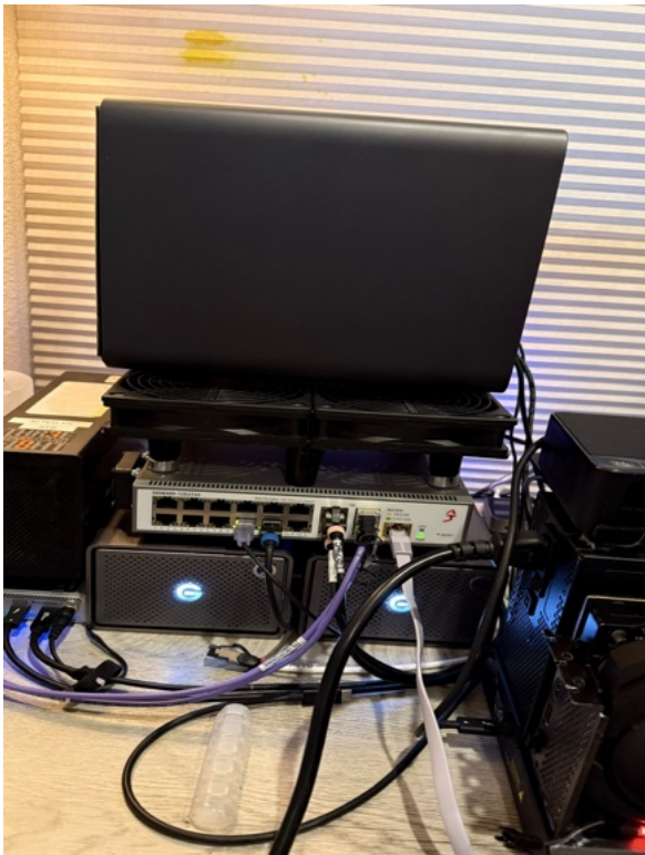
Multiple GPU's, a Custom Configured Minisforum N5 Pro Network Attached Storage with Integrated AI Computer Running Ubuntu with an External eGPU RTX GeForce 4070 Ti Super OC via OcuLink, Running OpenClaw w/ a Host of Agents for Legal Document Creation, Multiple SSD's + Enclosures, 10G Fiber, Switch, & More...
