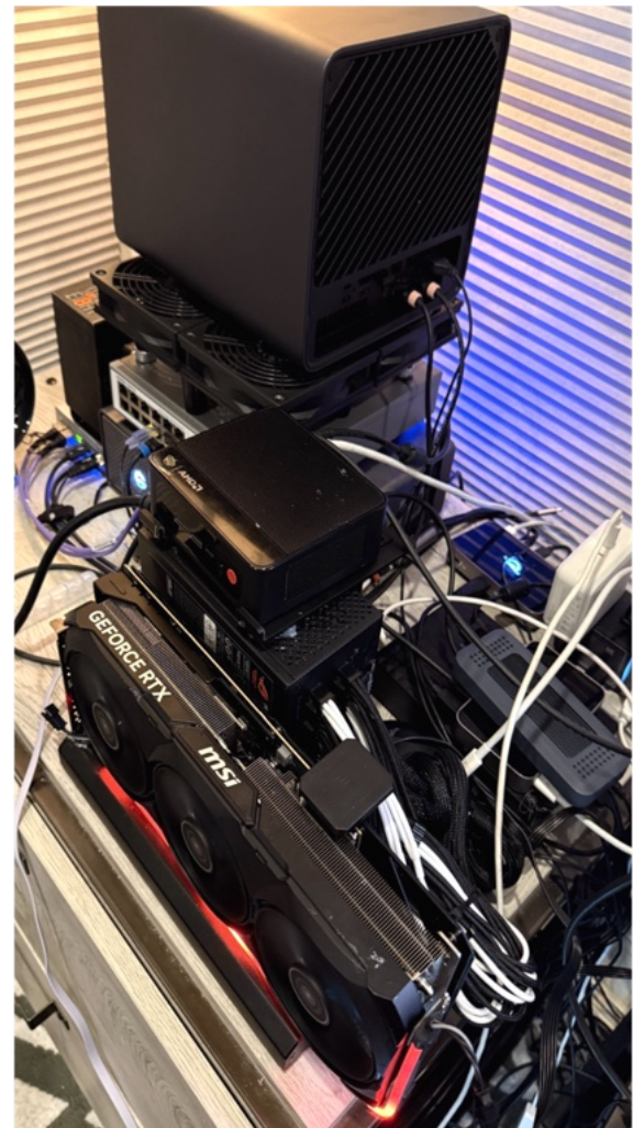
Multiple GPU's, a Custom Configured Minisforum N5 Pro Network Attached Storage with Integrated AI Computer Running Ubuntu with an External eGPU RTX GeForce 4070 Ti Super OC via OcuLink, Running OpenClaw w/ a Host of Agents for Legal Document Creation, Multiple SSD's + Enclosures, 10G Fiber, Switch, & More...
